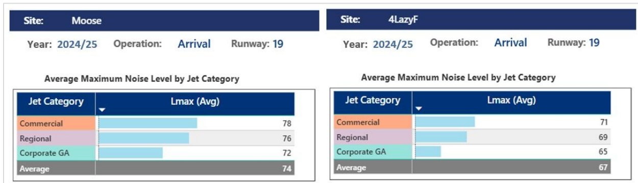
Figure 5: Measured Single Event Noise Levels (2024/2025)
