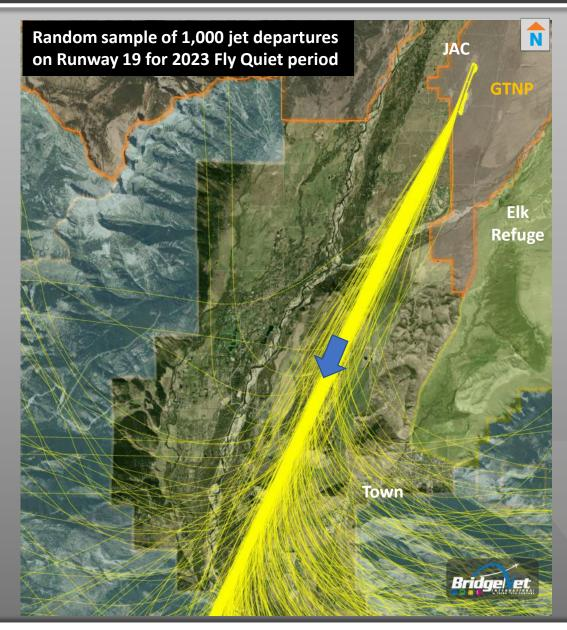
Use of aircraft flight management system (FMS) computer reduces westward drift on south departures
