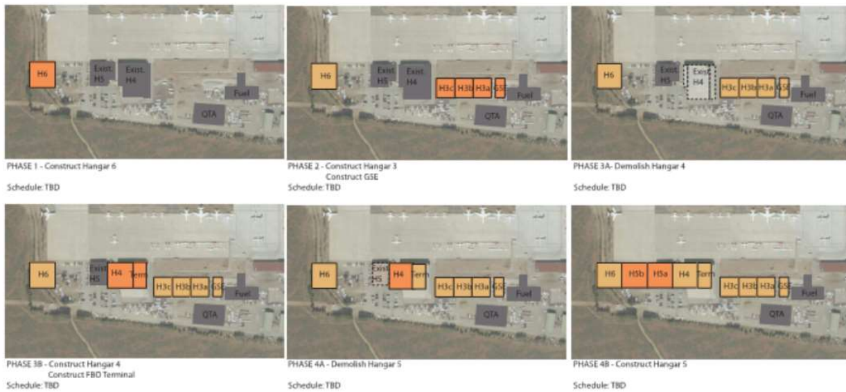
Figure 21. Construction Phasing Plans
